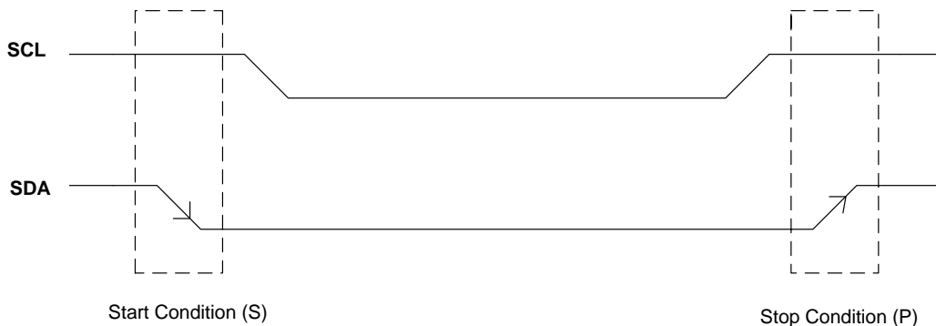
Figure 1. I 2 C Start and Stop Condition
